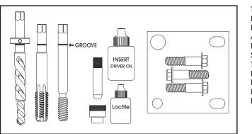
Tools needed: Drill fixture Drill bushing Alignment pin Bolts (3) Step drill Tap Insert driver Inserts (10) loctite Driver oil
