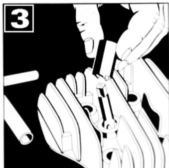
Use WD40 for cutting or grease to help catch chips.
