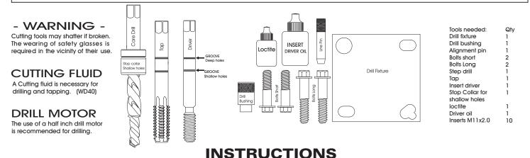
The NorthStar 2004 has 2 depths of holes, shallow on the upper bank are 29mm.
