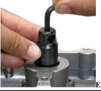
Oil the bottom threads of the insert driver with a few drops of driver oil. This can also be 30wt motor oil While screwing the driver into the insert you will feel the driver start to tighten up, with a little more power continue through the insert
